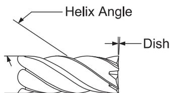
**Helix Angle** – Varies from 0 to 60 degrees. Higher helix angles can increase the number of teeth in a cut, and help in redirecting cutting forces. This is beneficial in harder to machine materials in particular. Changes in helix angle can also greatly affect the flute form of an end mill, and affect chip evacuation.
