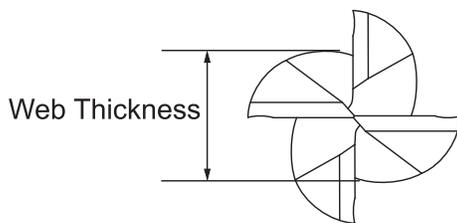
**Web Thickness** – The cross section of the fluting of the end mill. Larger webs allow for more rigidity, while smaller webs allow for better chip evacuation. This feature is highly dependent on the material being machined.
